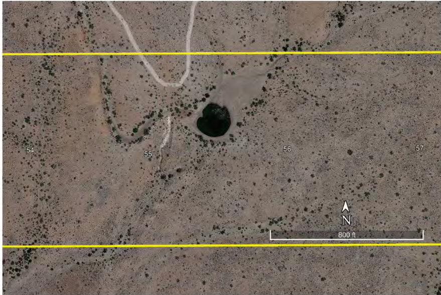
Figure 5. Standing water 275-325 feet east of structure 55 and west of structure 56. Yellow lines indicate the CEC corridor. White numbers indicate structure locations.
